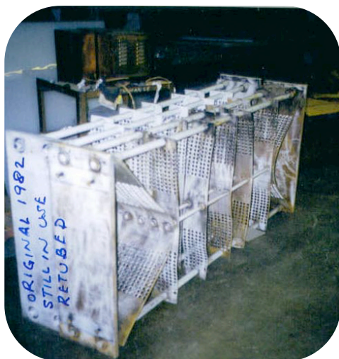
Original Heat Exchanger
